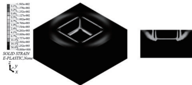
图11 既有支护桩排边角处失稳时土体塑性应变云图 Fig.11 Plastic strain contour of soil mass during failure at corner position of existing support row pile
